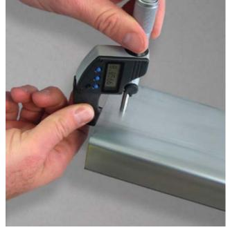
ber, and twist. Measurements will be taken to verify all steel properties; including mil thickness, yield strength, and coating weight (actual zinc coating weight per surface area). CSSA upholds the most current standards in accordance with IBC 2012.
